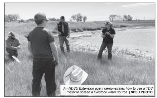
and easy to use. If the screening indicates the TDS is greater than 4,500 ppm and/or sulfates are greater than 800 ppm, submit a sample to a lab for additional analysis.
